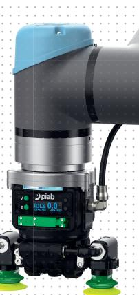
Piab's piCOBOT® mounted on a UR collaborative robot designed to act as a flexible co-worker in a variety of production, packaging or assembly lines.
